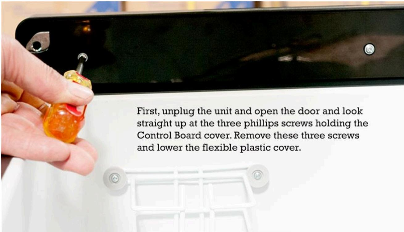
First, unplug the unit and open the door and look straight up at the three phillips screws holding the Control Board cover. Remove these three screws and lower the flexible plastic cover.
