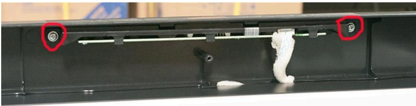
Now you will see the Kegerator Control board secured with two phillips screws. Remove these and pull the board down gently.
