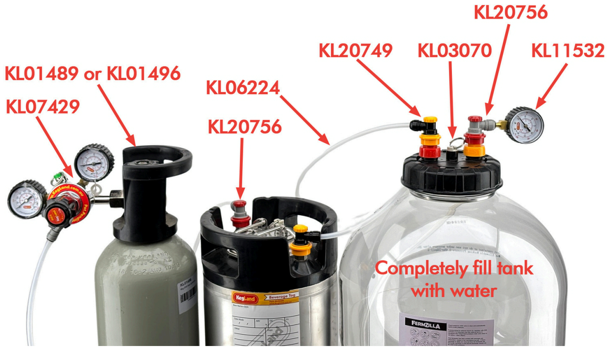
Hydro Test - Cornelius Keg Setup
