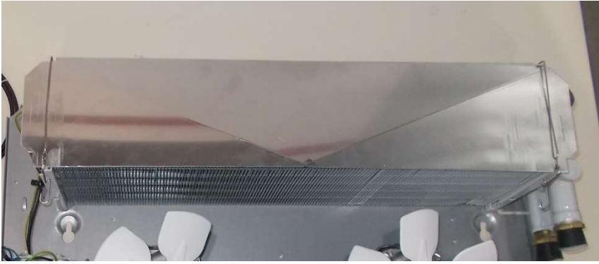
2.5 Mount the defrost water sheet
