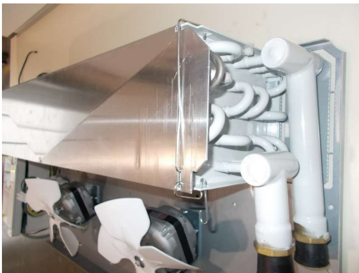
2.6 Fix it by using the fastening clips
